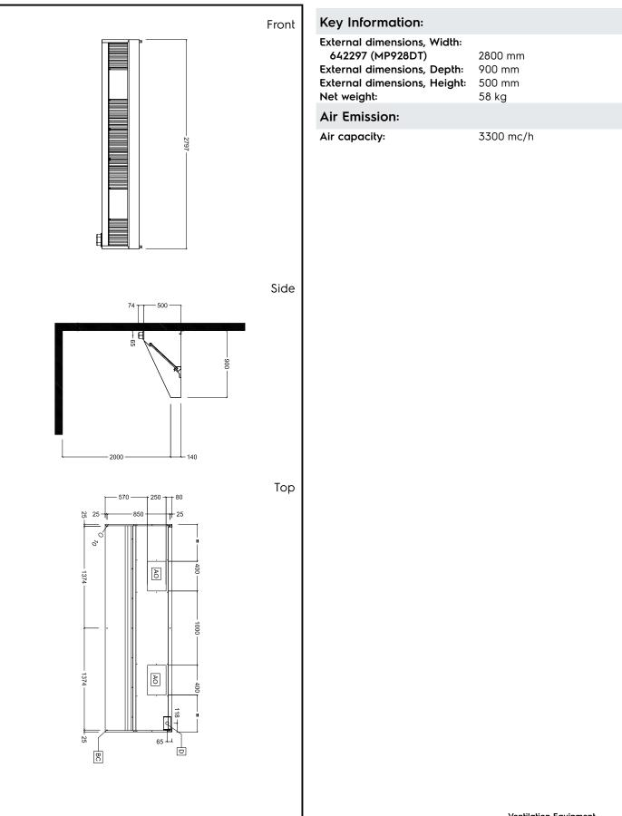
Ventilation Equipment 304 S/S Wall Hood+Filters 2800X900mm
